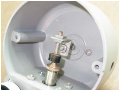
Standard Invalco control (bracket up)
