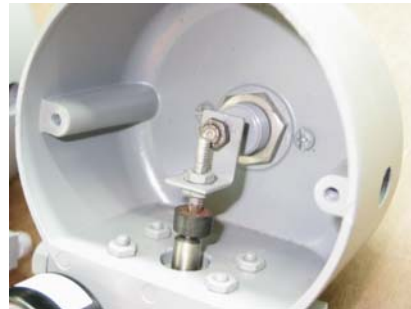
Invalco control with Mizer (bracket down)
